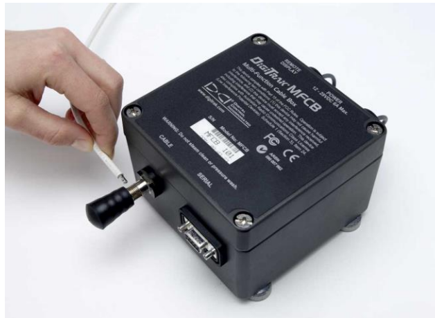
Connecting Transmitter Cable to Cable Box
