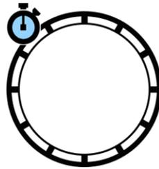
An expired User Code will not stop the receiver from functioning; this only happens if the Master Code expires. However, the stopwatch icon alerts the operator that use is subject to the Master Code timer. To prevent the alert, instruct the operator to enter the User Code regularly, such as every morning or every Monday.
