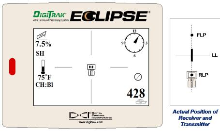
Eclipse Locating Display with Target in Box at RLP
