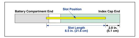
Standard and Dual-Frequency Transmitter Housing Slot Requirements
