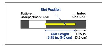
Mini Transmitter Housing Slot Requirements
