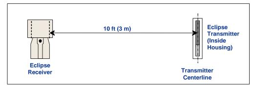
10-Foot Measurement for 1-Point Calibration
