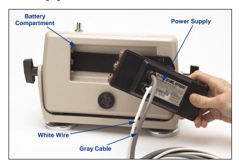
Insertion of Power Supply in Remote Display
