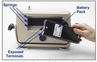
Installing Battery in Remote Display
