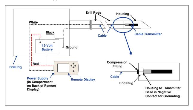
Connecting Cable System Components
