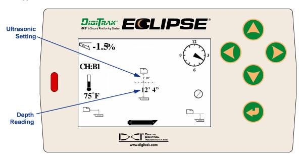
Depth Screen on Remote Display (when receiver is above LL)
