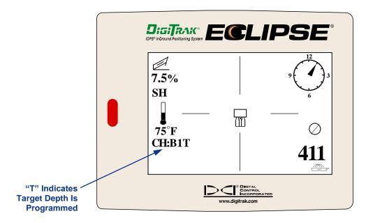
Receiver Screen with Target Depth Programmed
