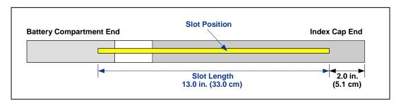
**Extended Long-Range Transmitter Housing Slot Requirements**
