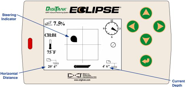
Target Steering Screen on Remote Display
