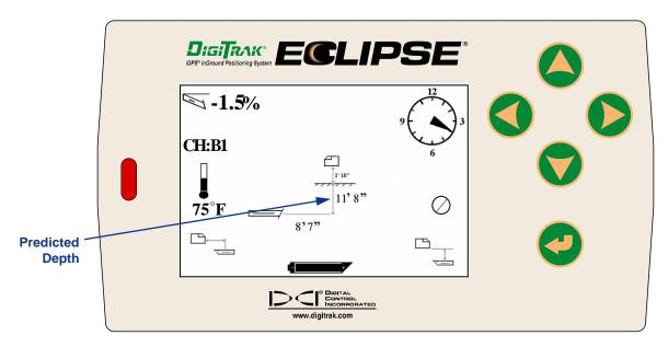
Predicted Depth Screen on Remote Display (when receiver is above FLP or RLP)
