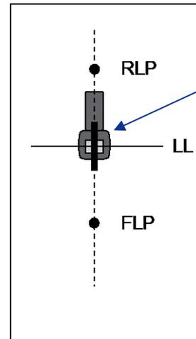
With the LL aligned in the box, the receiver may face toward the RLP or FLP during depth readings.
