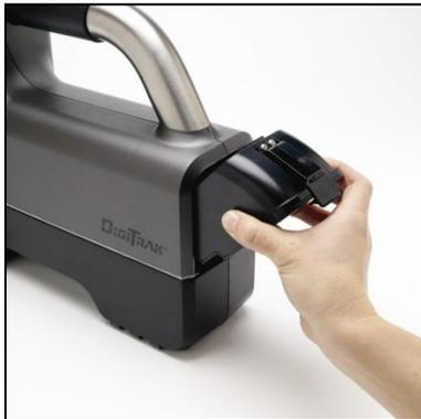
*Inserting Battery Pack*
