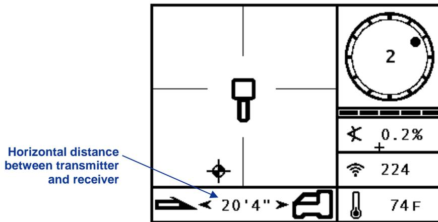
*Receiver Screen with Target Depth Programmed*
